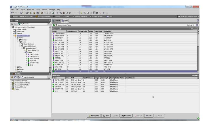
Single or multiple points can be added as control points with System600ProxyExt extensions by selecting the discovered row(s) in the top pane, and clicking add. Doing so will cause the "Add" dialog box to appear:
